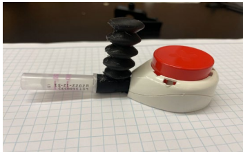
Figure 4: A modified Tasso device with an extra vacuum chamber to attempt to draw out more blood.
