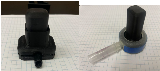
Figure 6: fully 3D printed vacuum blood extraction devices with (left) a rectangular base and (right) a circular base to better adapt to placement on sheep ears.
