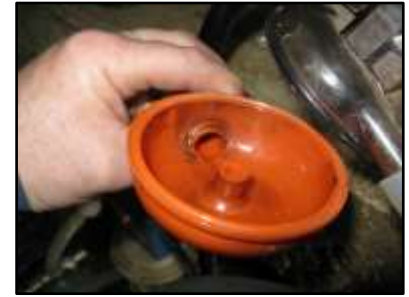
Fig. 13. Inking from rubber breakdown
