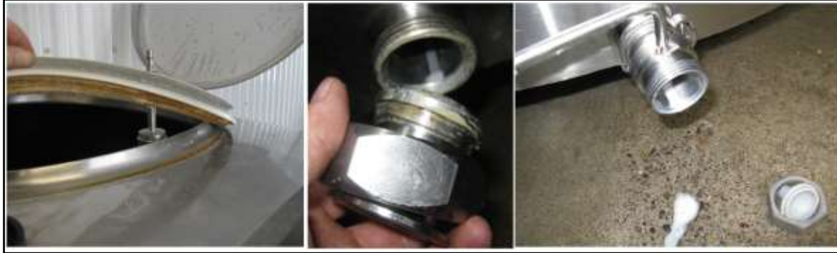
Fig. 16 Milk tank equipment needs to be inspected and cleaned after every pick-up
