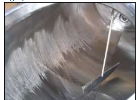
Fig. 15 Check tank for milk residues
