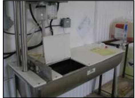
Fig. 19 Covered wash sink helps maintain temperature of wash water
