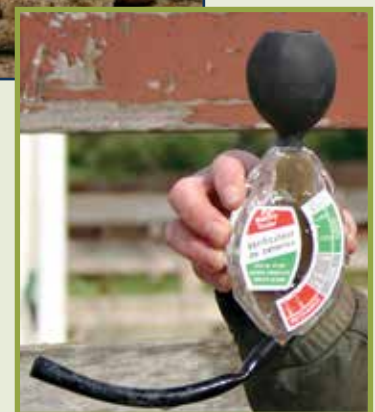
Above: Footrot treatment is time-consuming, expensive and back-breaking work. Right: Check the zinc sulphate concentration using a battery tester.
